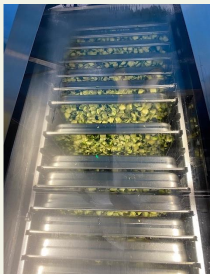
Photo 2 & 3: The industrial washer in action: used for hygienically cleaning the stainless steel food containers from public kitchens (Source: L'EntrePôt)
